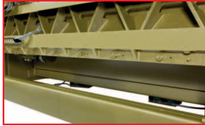
Lardone deformabile. Adjustable gib for blade cylinder.
